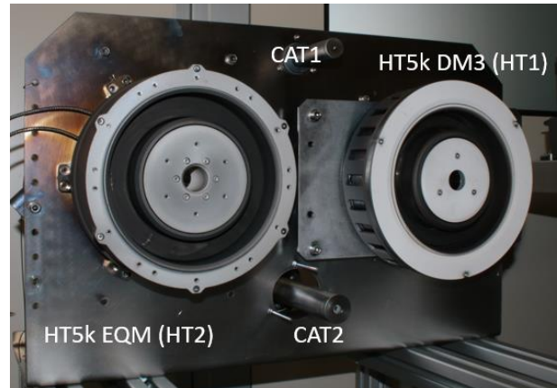
Figure 12. HT5k thrusters used for the EDDA test. On the right, the HT5k DM3 (HT1), on the left the HT5k EQM (HT2).
